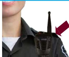
**Emergency:** A confirmation beep sounds when pressed\*# and then triggers host radio's emergency function. Press button as per mobile radio's emergency operating instructions or as advised by your supplier.
